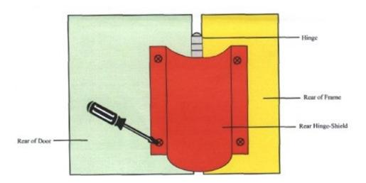
Remove the protective coating from the tape. Line up the edge of the rear hinge GUARD parallel to the guideline on the frame. Press firmly to hold in position before finally securing with the <u>screws</u> provided (the screws should be fitted at approximately 300mm centres). Repeat this procedure to attach rear hinge GUARD to the door
